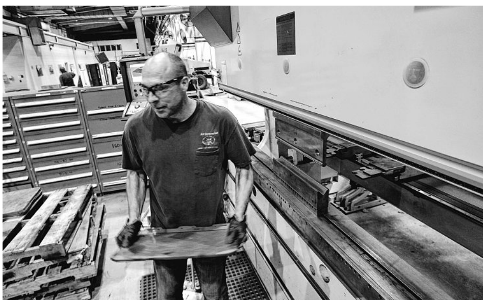
Laser operator Brian Hamilton uses a press brake to bend 3/8-inch armor plates with 100 tons of force at the Army Prototype Integration Facility at Picatinny Arsenal. BOB KARP/STAFF PHOTOGRAPHER
